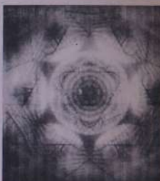
Zone axis pattern for a single silicon crystal
